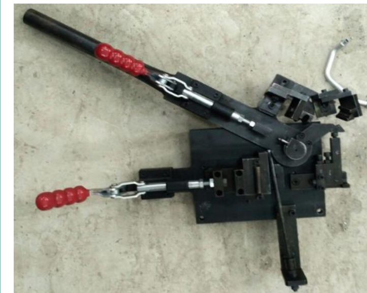
ALUMINIUM PIPE BENDING FIXTURES
